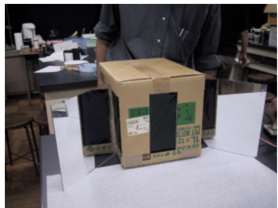
Figure 3. Three colors mixing box by using two mirrors
